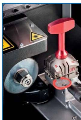
Flat and cruciform key cutting station
